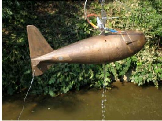
Abbildung 3-3: US – P61 Suspended Sediment Sampler
